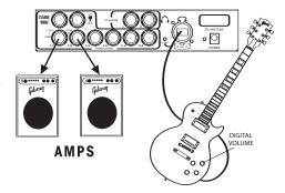
HEX output — each string with its own output. This connection requires six separate analog audio inputs such as six amps or a PC audio card with six inputs. Plug each analog input into one of BoB's FROM GUITAR output jacks (1-E through 6-E).
