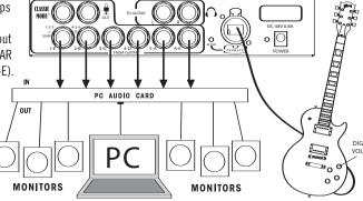
3. Connect your guitar to BoB. Plug one end of the Cat-5 cable into the guitar's MaGIC jack and the other end into BoB's MaGIC jack. The Neutrik Ethercon locking connectors were designed to maintain a connection, without signal breakup, under typical guitar playing conditions.
