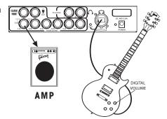
STEREO output — 2x3 separation with EAD (lower pitched) strings through one amp and GBE (higher pitched) strings through a second amp. Plug the cord from the amp for the EAD strings into BoB's 2-B FROM GUITAR output jack (also labeled 4-5-6 R). Plug the cord from the amp for the GBE strings into BoB's 1-E FROM GUITAR output jack (also labeled 1-2-3 L).
